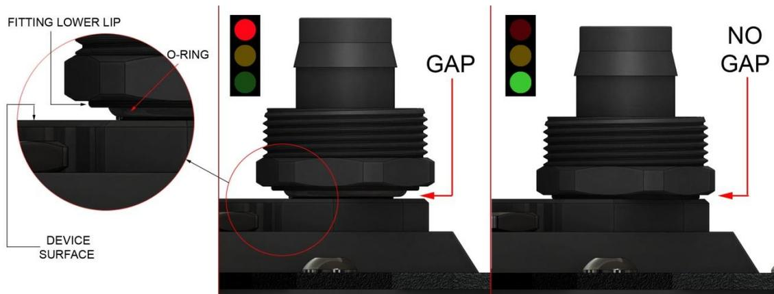
(\*) The amount of force necessary to screw the fittings down in “finger tight” mating position may substantially vary from one device to another depending on various factors. Users are advised to always visually check on the actual position of the fitting relative to the device surface rather than solely relying on feel. There should be little -not to exceed the thickness of a sheet of paper, or no visible gap between the fitting lower lip and the device surface.
