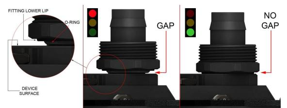
(\*) The amount of force necessary to screw the fittings down in "finger tight" mating position may substantially vary from one device to another depending on various factors. Users are advised to always visually check on the actual position of the fitting relative to the device surface rather than solely relying on feel. There should be little -not to exceed the thickness of a sheet of paper, or no visible gap between the fitting lower lip and the device surface.
