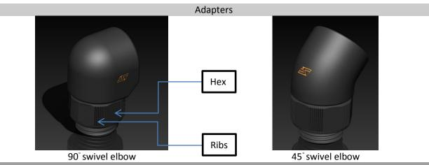
All Lok-Seal<sup>™</sup> adapters (swivel or non-swivel) feature a combination of finger grip ribs, as well as a hex shape so they can be easily and properly secured to your cooling devices. A choice of 2 common tools can be used: adjustable wrench or 17mm Metric flat wrench.
