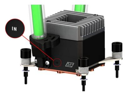
Attach the tubes to the hose-barbs, and secure them with the provided hose-clamps. The water-block inlet is specific, and indicated by an "IN" marking on the side of the waterblock housing.
