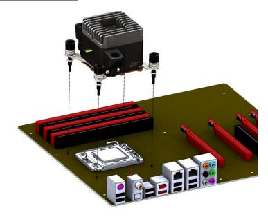
Lower the Apogee<sup>™</sup> Drive II onto the CPU, and align the spring loaded screws with their respective mounting holes. Then fasten the screws alternatively and in a cross-pattern until they bottom out. The Apogee<sup>™</sup> Drive II can be installed in any orientation with respect to the socket.
