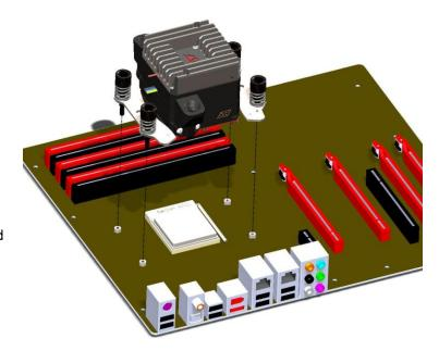
Lower the Apogee™ Drive II onto the CPU, and align the spring loaded screws with their respective mounting holes. Then fasten the screws alternatively and in a cross-pattern until they bottom out.
