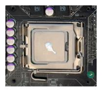
Clean the CPU with a degreaser (preferably formulated for electronics) then apply the supplied Tim-Mate thermal compound.
