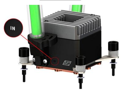
Attach the tubes to the hose-barbs, and secure them with the provided hose-clamps. The water-block inlet is specific, and indicated by an "IN" marking on the side of the waterblock housing.
