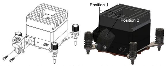
The inlet and outlet ports are installed straight up by default. They can also be installed at an angle to facilitate tube routing. To change the orientation of a port, loosen the 2 screws holding the port to the waterblock body and rotate the port until the holes match those in the waterblock, and then re-insert the existing screws.
