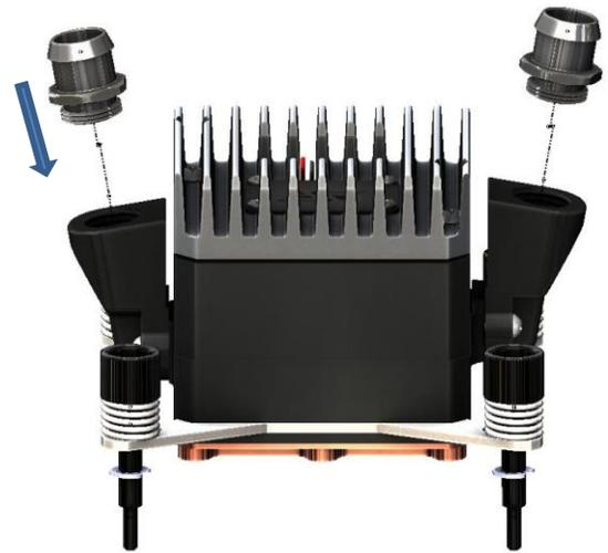
Install the provided barb fittings – Fasten the fittings by hand until they mate with the port surface. Then lock them in place with an extra  $\frac{1}{4}$  of a turn using a  $\frac{5}{8}$ " tool (flat wrench or socket wrench).
