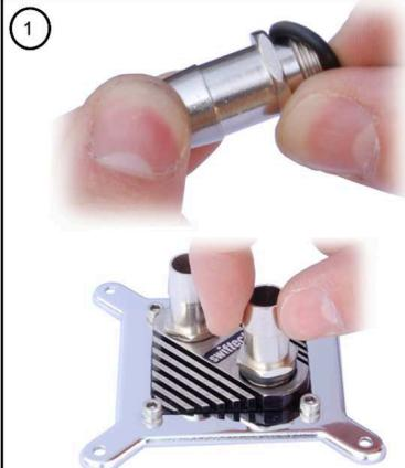
**UK** 1 set of 1/2" barb fittings is supplied (3/8" fittings are available in option). Install the o-rings and fasten the fittings to the water-block, making sure to give them a firm lock.
