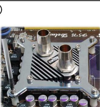
**UK** Tighten the 4 screws in the 4 nuts alternatively and gradually. Done!
