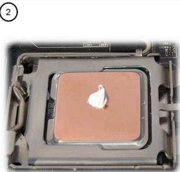
**UK** Remove the existing heatsink from your motherboard, clean the CPU with a xylene (degreaser) based cleaner then apply the Arctic Céramique thermal grease to the CPU (look at the picture).
