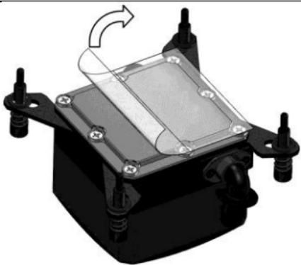
Remove the protective plastic cover from the CPU cooler.
