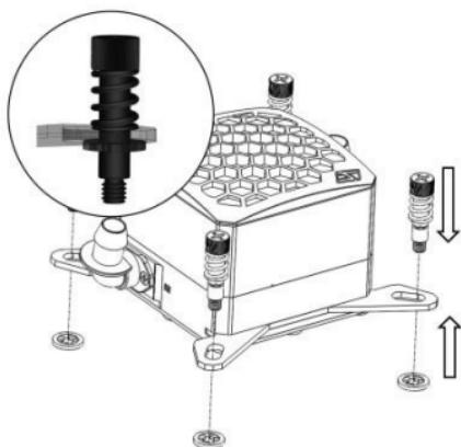
Install the provided Intel® LGA 2011 spring-loaded screws.
