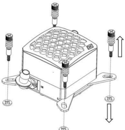
By default, the CPU cooler is shipped with Intel® LGA 1366/1155/1156/775 spring-loaded screws pre-installed.
