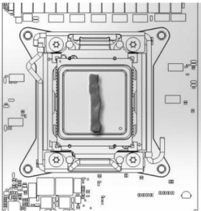
Clean the CPU with a degreaser (preferably formulated for electronics) then apply the supplied TIM-MATE 2 thermal compound across the processor as shown.
