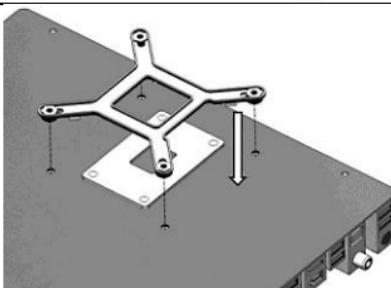
Mate the back-plate to the back of your motherboard, making sure that the standoffs are correctly inserted into the motherbard holes. Your motherboard is now ready for installation of the CPU cooler.
