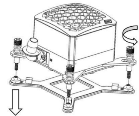
For the purpose of protection from shipping damages, the CPU cooler is shipped with the universal motherboard back-plate pre-installed. It needs to be removed first.
