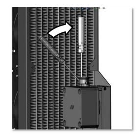
6. Finally, while firmly pushing down on the top of the screw driver to maintain it in place, firmly fasten the remaining screw till it bottoms out. This is not particularly easy, and requires a good grip since the screw driver is small and offers little holding surface. You may also use a pair of thin nose pliers (instead of your fingers) to get a better grip on the screw driver and lock the screw into place.
