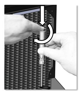
Inspect that both screws are fully tightened and make sure that there is no gap between the fitting and its mating surface or it will leak! You are done!
