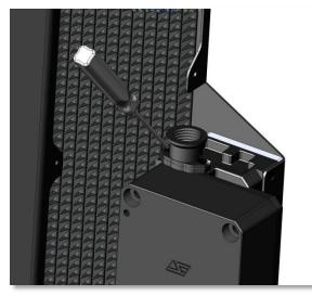
...And then straighten the screw driver. The shaft of the screwdriver may bow a little, since there is so little space
