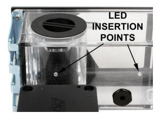
Apply a small drop of cyanoacrylate type of glue (Loctite, Superglue, Krazy glue) (not provided) to the LED body, and immediately insert it in one of the desired holes. We recommend testing the illumination (with coolant) of your preferred location prior to gluing the LED.
