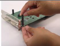
Screw the female-female threaded standoff over the PCI bracket
