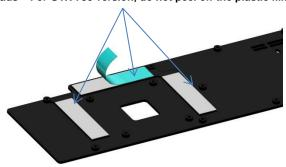
5. Peel-off the protective plastic film from the waterblock thermal pads
