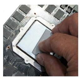
Apply the provided Arctic Céramique thermal paste to the GPU heat spreader as shown above.
