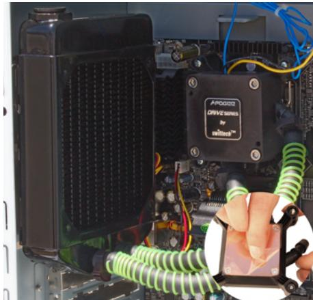
4. Fasten the Apogee™ Drive to the processor by tightening all four screws progressively and in a cross pattern until you reach a firm positive lock. Cycle thru the four screws twice to make sure that you have equal tension on all four.
