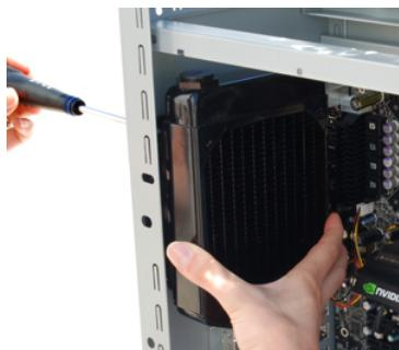
Fasten the screws just enough to hold the radiator in place.
