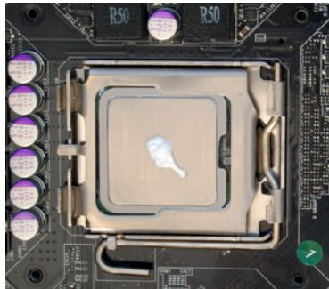
1. Apply the provided Arctic Céramique™ thermal grease at the center of the CPU as shown above.
