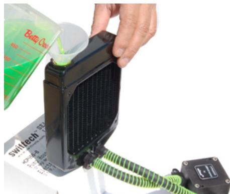
Place the system on your bench table, with the radiator positioned higher than the pump and pour coolant into the radiator fill-port until full.
