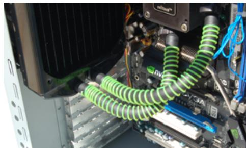
3. Adjust the second tube to the radiator, cut it to length then push the tube onto the fitting.
