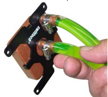
Figure 7 Purge the air from the water-block, by pointing the discharge spigot upwards
