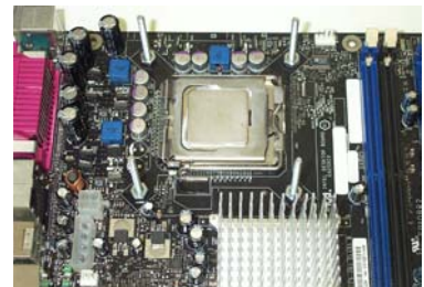
Figure 6 Install retention posts
