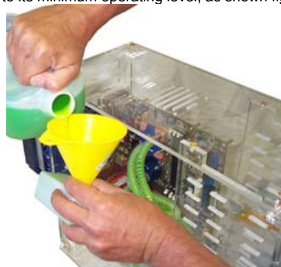
Figure 4: If possible or desired, you can also fill the reservoir outside of the chassis. Tipping it steeply at an angle will allow you to fill-it up at the maximum operating level as shown figure 5. Do not forget to close the fill-cap before you re-install the unit into the drive bay!
