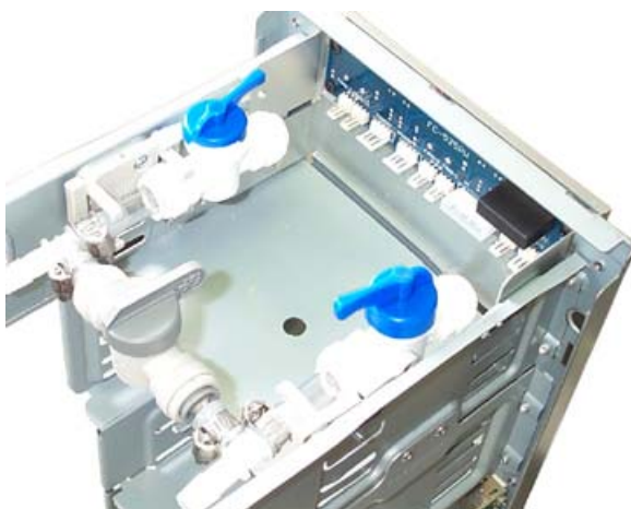
Figure 2 - Notice how the ball valves are only held by one set of jaws in this example.
