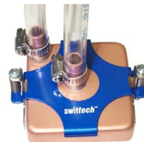
Figure 3 - Tubes attached with worm-drive clamps
