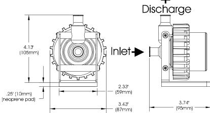
Do not utilize small diameter or flow restrictive fittings in the pump inlet line. Minimum line inner diameter is 3/8". An example would be a reservoir with 1/4" fittings. This will cause the pump impeller to cavitate, lose prime, stop pumping and damage the pump (see warranty note \*\*\*).
