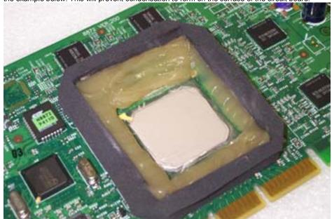
d. Lightly coat the GPU with the provided thermal compound. Only a paper-thin coat is necessary. It should be applied using preferably a razor blade, or a credit card, held between thumb and index at a 45-degree angle.
