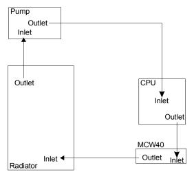
e. Re-install the graphics card in the AGP slot, and proceed with filling and bleeding the cooling circuit. A mix of 75% purified water and 25% antifreeze is recommended
