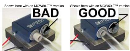
Make sure that the tubes are fully inserted into the fitting. The tip of the plastic tube inserts should be flush with the inlet and outlet openings, as shown above. Inserting the tubes requires a firm push, accompanied by a twisting motion, and a little bit of grease around the tubing really helps <sup>(i)</sup>
