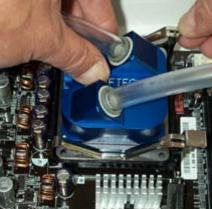
Step 1 Position your block inside the retention frame. Put both clips in place for the next step, by simply slipping the hook of each clip into the holes of the retention frame. Step 2 While maintaining the opposite side of the block to prevent it from tipping over, push down on the clips' thumb-tab until the hook catches the hole in the retention frame. Step 3 Keep maintaining pressure on the block to prevent it from tipping over, and hook-down the second clip. Installation is complete!
