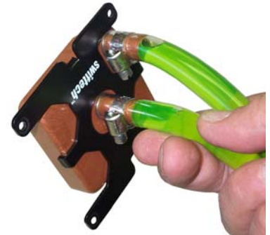
Figure 3 Purge the air from the water-block, by pointing the discharge spigot upwards
