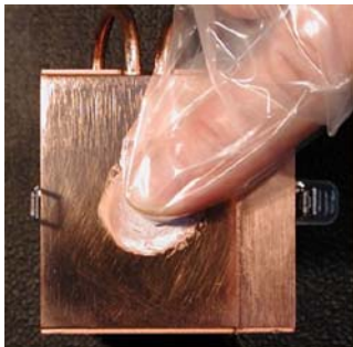
Rub some compound in base of water-block first, and then clean off with lint-free cloth.
