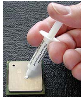
Apply small amount of compound on the CPU heat spreader
