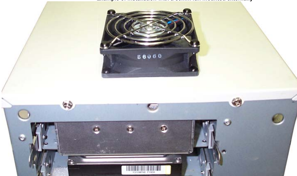
Example of installation with a 80mm fan mounted externally
