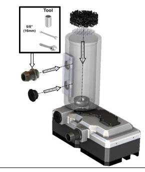
Attach your tubing, and secure it with the provided hose clamps. Then, fill-up the reservoir being careful NOT TO SPILL COOLANT ON THE PUMP (see warranty notice below), and finally <u>firmly</u> fasten the cap by hand making sure that the O-ring remains located inside of its groove (so it doesn't get pinched).
